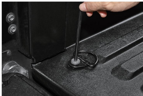
24. Remove the D-ring tie-down at the rear corner and set it aside for later use. Note: The washer inside the mounting hole can be left in place.
