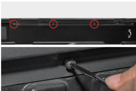
51. Remove the three original screws marked in red on the top and set them aside for later use.
