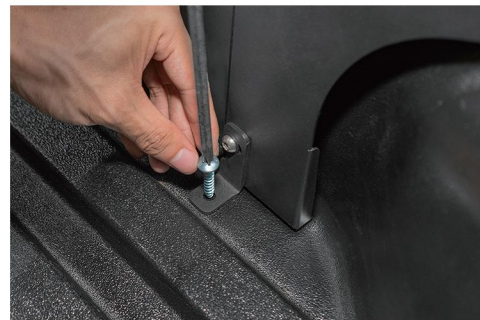
58. Use a Phillips screwdriver to fasten the self-tapping screw ⑮ into the vehicle body.
