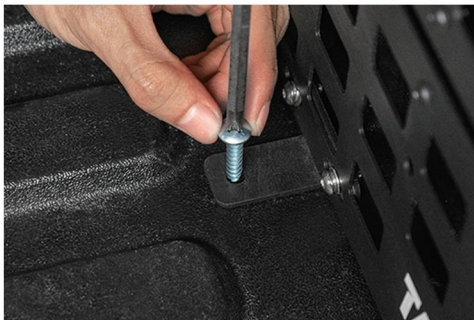
21. Use a Phillips screwdriver to fasten the self-tapping screw ⑮ into the vehicle body.
