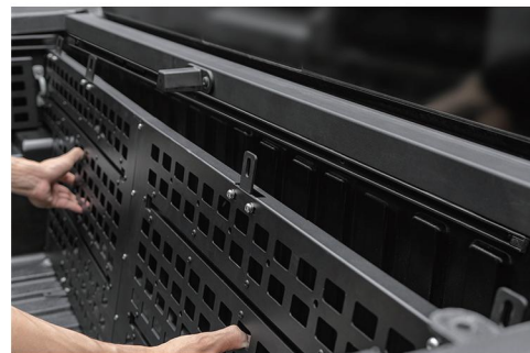
19. Insert the ⑤-⑥ assembly and align the bottom ⑪ with the groove.
