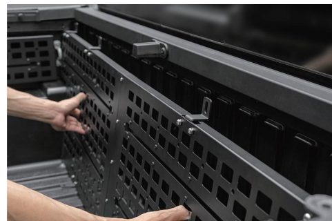
46. Insert the ⑤-⑥ assembly and align it with the original mounting holes, then align the bottom ⑪ with the groove.
