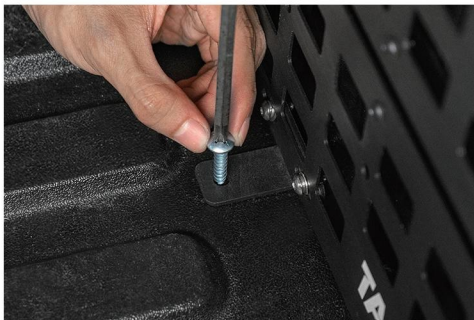
48. Use a Phillips screwdriver to fasten the self-tapping screw ⑮ into the vehicle body.
