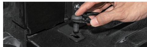
52. Remove the D-ring tie-down at the rear corner and set it aside for later use. Note: The washer inside the mounting hole can be left in place.
