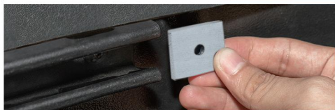
26. Remove the end cap from slide rail and insert three ⑫, then reinstall the cap. Note: Remove any other components from the rail before proceeding.
