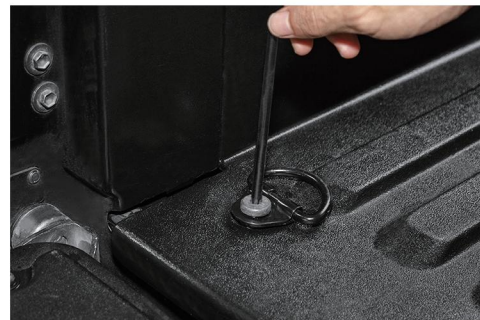
52. Remove the D-ring tie-down at the rear corner and set it aside for later use. Note: The washer inside the mounting hole can be left in place.
