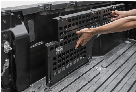
54. Insert the ①-② assembly. Align with the mounting holes of front corner tie down hook and rear corner D-ring tie-down.
