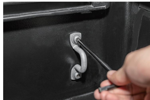
25. Remove the tie-down hook at the front corner and set it aside for later use.
